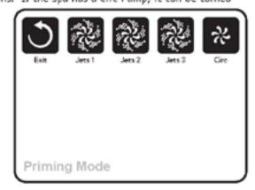
the pumps and repeat the process. Note: Turning the power off and back on again will initiate a new pump priming session. Sometimes momentarily turning the pump off and on will help it to prime. Do not do this more than 5 times. If the pump(s) will not prime, shut off the power to the spa and call for service.
